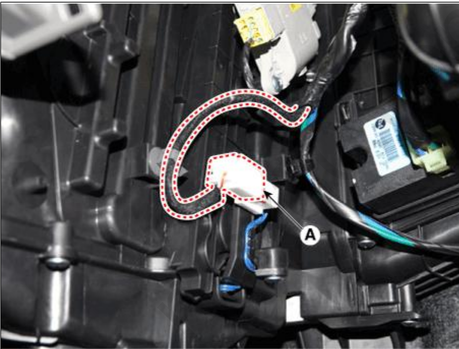
(6) Disconnect the intake actuator connector (A).
